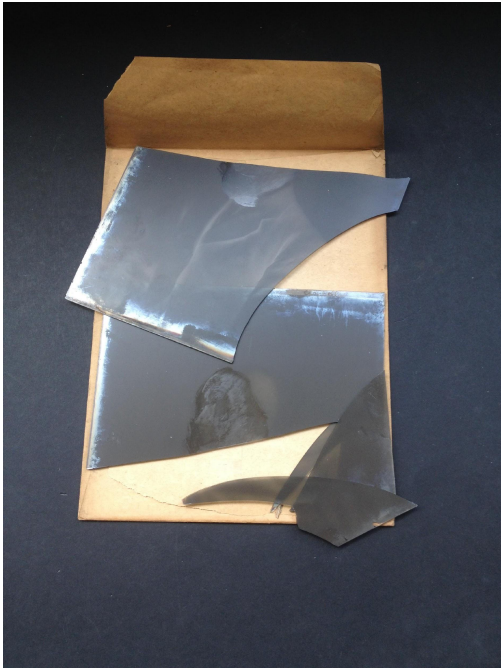
Damage to plates caused by damp & collapse of shelves: breakage, cracking, delamination, blocking
